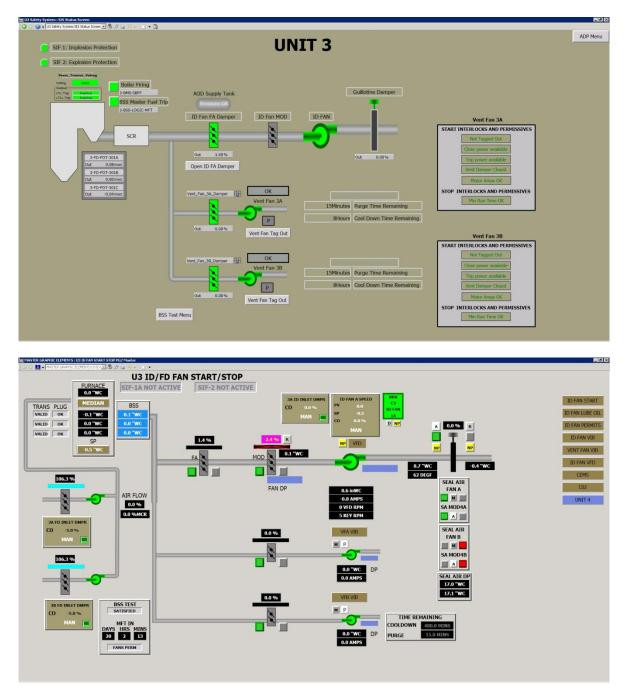
Whenever a SIF (Safety Instrumented Function) is actuated, the boiler will have been tripped already. As a result, the method we determined would be best to reset a SIF was to proceed through the off-line testing required prior to a boiler pre-purge. This would then reset the SIF and allow normal operation.
